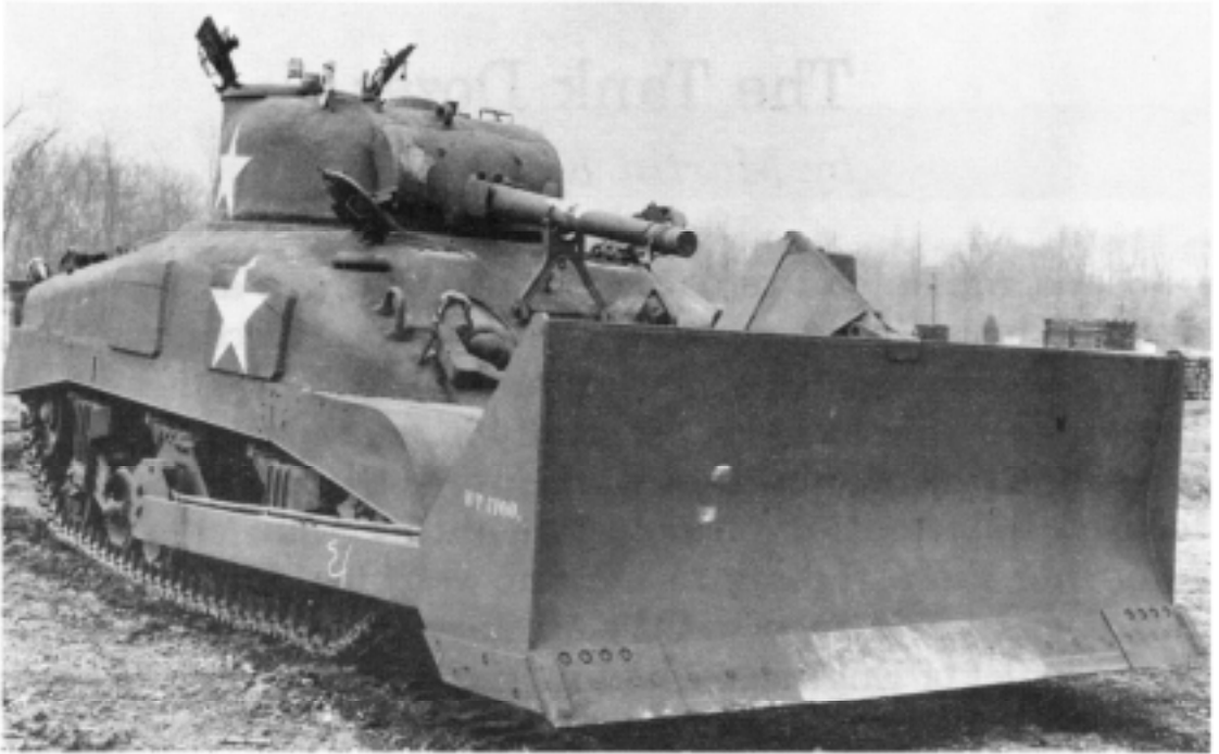
The tank dozer could plow a path through dragon's teeth and antipersonnel obstacles found on invasion beaches.
