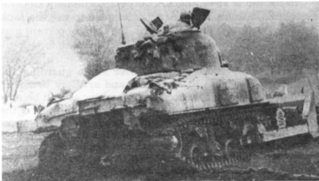
The tank dozer smooths the way as soldiers of Company C, 23d Armored Engineer Battalion, demonstrate obstacle breaching techniques on the Siegfried Line, 1944.
