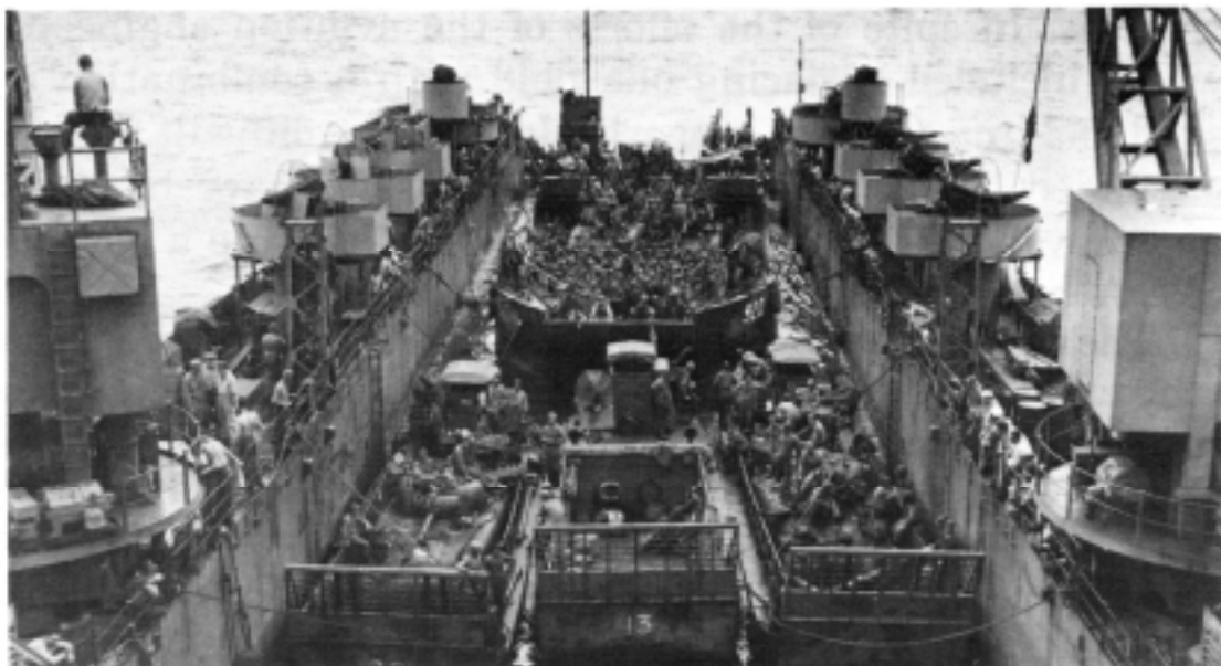
Engineer LCVPs and LCMs load into the well deck of a landing ship, dock, just before the Hollandia landings 22 April 1944.
