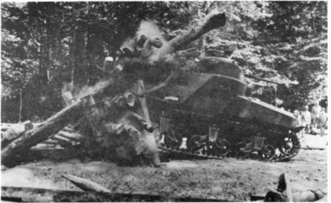
As part of their training at Fort Belvoir, Virginia, engineers test how well an obstacle can withstand a tank attack.
